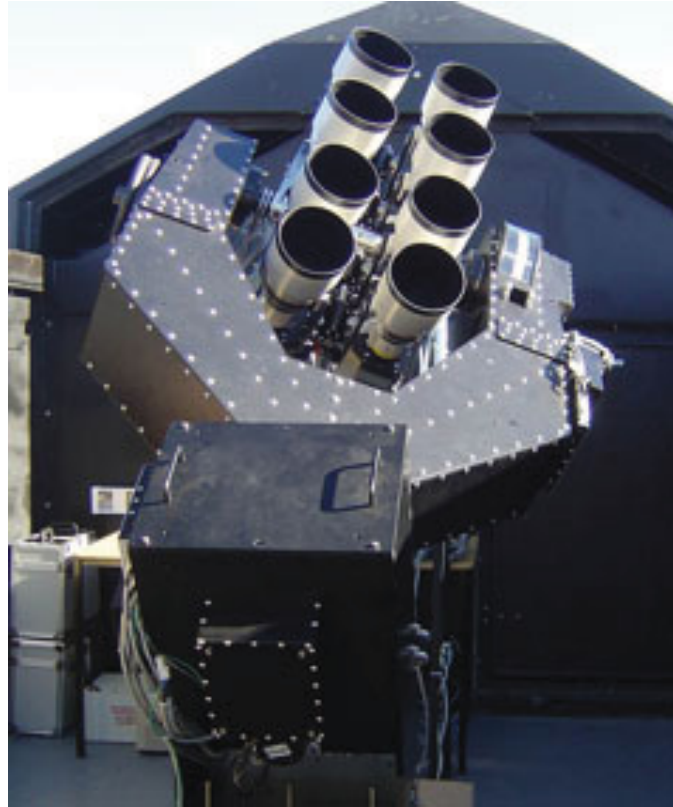
Figure 3.1.: SuperWASP-South Cameras. Eight telephoto lenses mounted on a single mount. Photo by David Anderson
