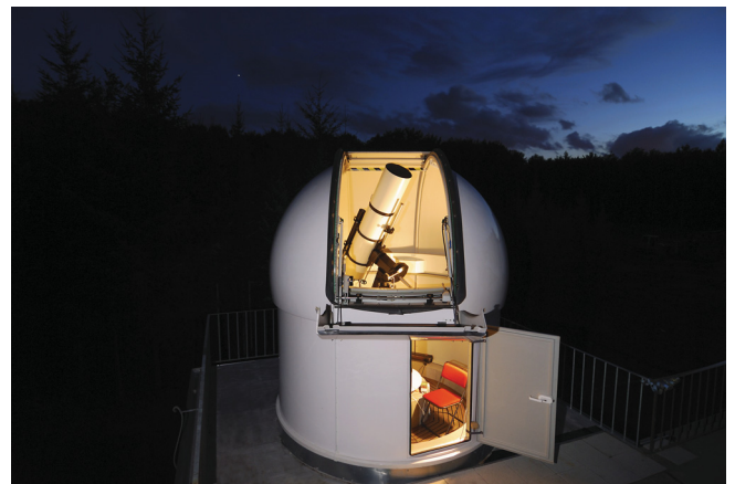
Figure 0.2.: The Tautenburg Exoplanet Search Telescope (TEST). A 30 cm aperture telescope with a square field of view with 2.2 degrees on each side.
